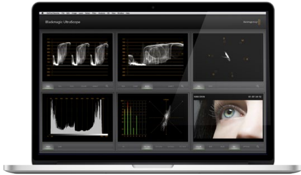
Blackmagic UltraScope - full screen view. Blackmagic UltraScope lets you accurately monitor the video and audio levels from your Blackmagic Cinema Camera or Production Camera 4K.
