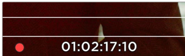
Blackmagic URSA indicates dropped frames by flashing the red "recording" icon at the bottom of the 10" LCD.
